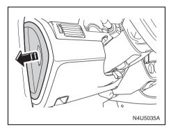
The instrument panel fuse block is located on the end of the instrument panel on the driver's side of the vehicle. To access the fuses, open the fuse panel door by pulling the door out.
